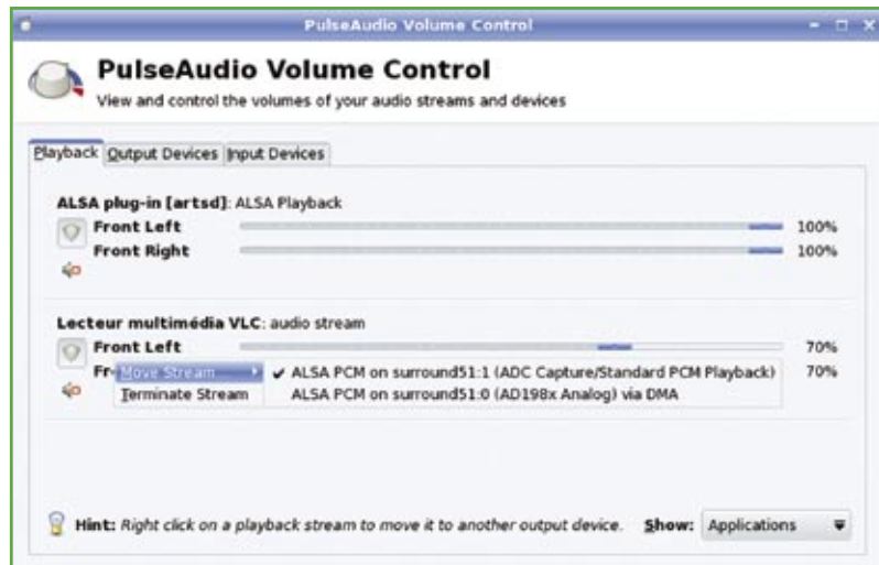
Figure 2. Moving on the fly the VLC audio flow. In order to complete this action, right click below the application name, select Move Stream and redirect to the desired output (the actual flow is indicated by the check mark located on the left of ALSA PCM... (ADC Capture...))
