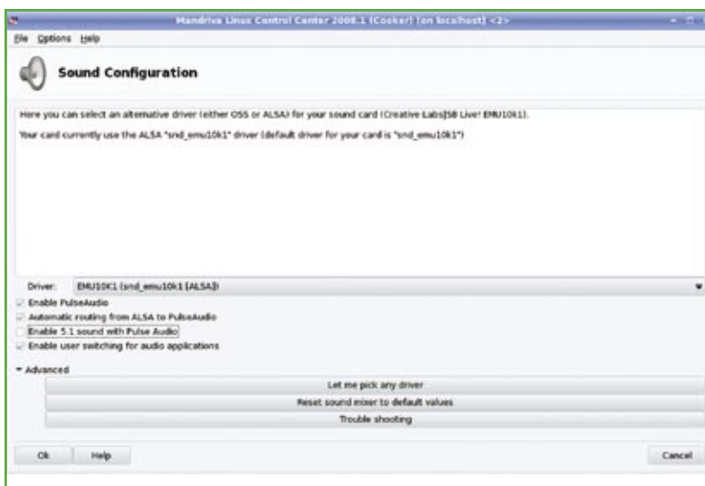
Figure 10. Activation and modification of the PulseAudio server behaviour from the graphical wizard draksound (available through the Mandriva Control Center at Hardware -> Sound Configuration
