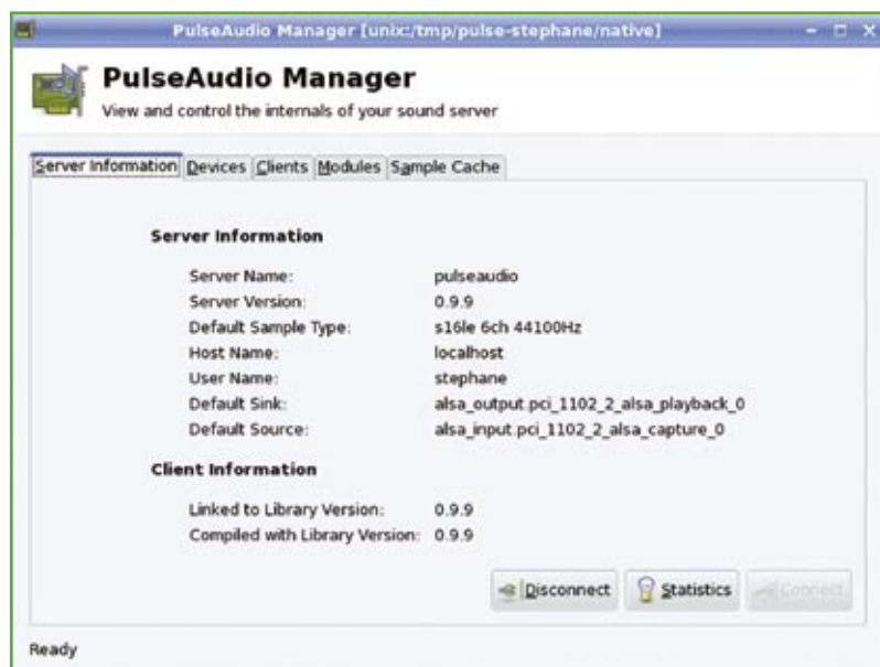
Figure 4. PulseAudio main control window. You will get the main server parameters in the first tab and in the other tabs, all the hardware and virtual devices managed by the server. This graphical manager should help you in controlling everything is in place and working as expected
